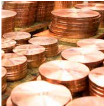
SEAM WELD WHEEL BLANKS
